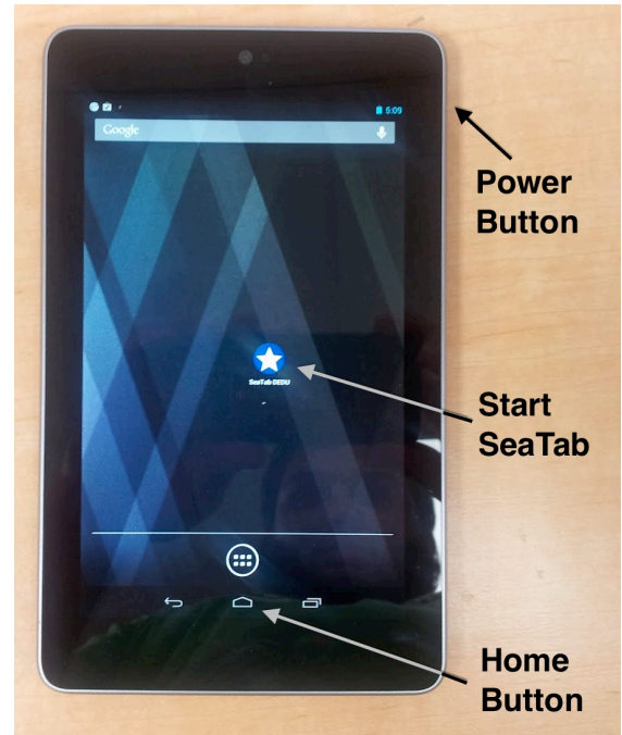
Figure 2. Google Nexus 7 tablet showing location of the hardware power button. Volume +/- buttons are directly below the power button. All other controls are in software.
