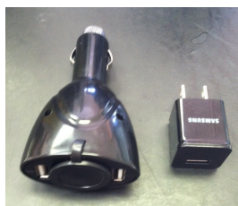
Figure 6. 12 VDC (left) and 120 VAC (right) to USB power converters.
