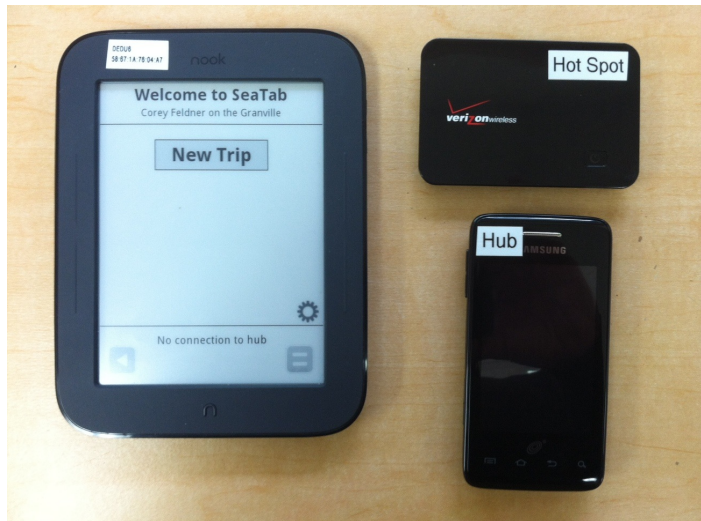
Figure 8. Components of the 3-device system: Barnes and Noble Nook, MiFi Hotspot, and Samsung Precedent.
